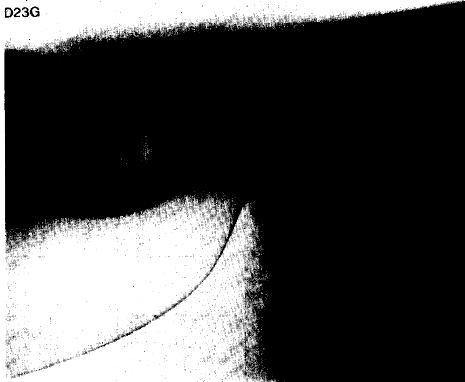
Fig. 4. TEM cross section of bird's beak formed using PELOX isolation.
