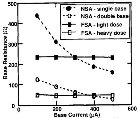
Figure 7 Base resistance as a function of base current for NSA bipolar transistors with single and double base contacts and FSA bipolar transistors with light and heavy extrinsic base implant doses.
