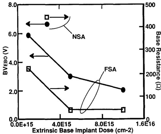
Figure 6 Base-emitter breakdown voltage and base resistance as a function of extrinsic base implant dose for bipolar transistors with 0.8X2.4µm emitters.
