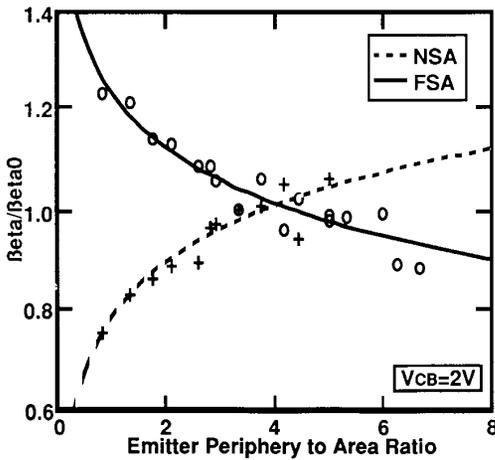
Figure 10 Normalized transistor gain as a function of emitter periphery to area ratio for FSA and NSA bipolar transistors.
