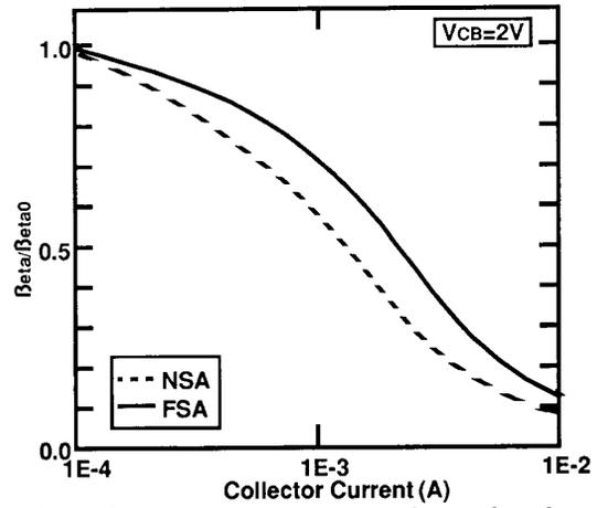
Figure 9 Normalized transistor gain as a function of collector current for FSA and NSA bipolar transistors with  $0.8 \times 2.4 \mu\text{m}$  emitters.
