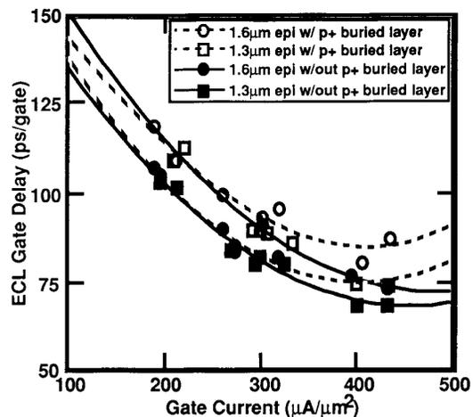
Figure 13 ECL gate delay as a function of gate current for fully self-aligned bipolar transistors with 1.3 versus  $1.6 \mu\text{m}$  epitaxial layer thickness and with and without  $p+$  buried layer. The FSA bipolar has a  $2E15$  extrinsic base dose.
