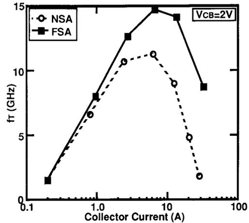
Figure 11 Cut-off frequency as a function of collector current for FSA and NSA bipolar transistors with  $0.8 \times 20 \mu\text{m}$  emitters.
