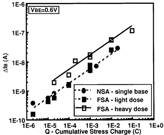
Figure 8 Increase in the non-ideal base current component as a function of cumulative stress charge during emitter-base reverse bias stress for FSA and NSA transistors with  $0.8 \times 2.4 \mu\text{m}$  emitters.
