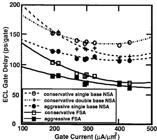
Figure 12 ECL gate delay as a function of gate current for NSA and FSA bipolar transistors with conservative and aggressive design rules. The FSA bipolar has a  $2E15$  extrinsic base dose.
