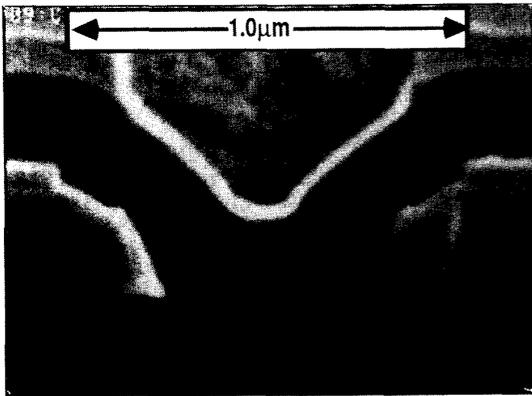
Figure 2 SEM Cross-section of double polysilicon, fully self-aligned bipolar transistor with a 0.4X1.2µm emitter.
