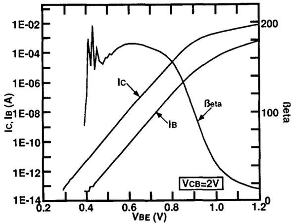
Figure 4 Gummel Plot of double polysilicon, fully self-aligned bipolar transistor with 0.4X1.2µm emitter.
