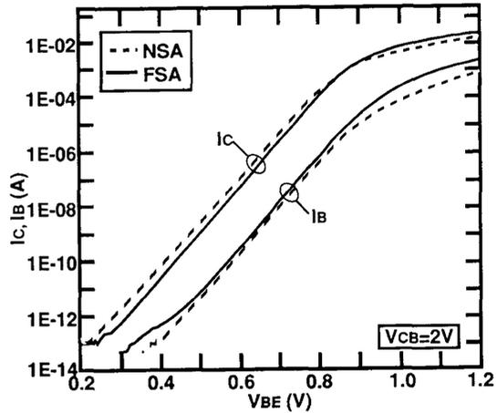
Figure 5 Gummel Plots for fully self-aligned (FSA) and non self-aligned (NSA) bipolar transistors with 0.8X2.4µm emitters.
